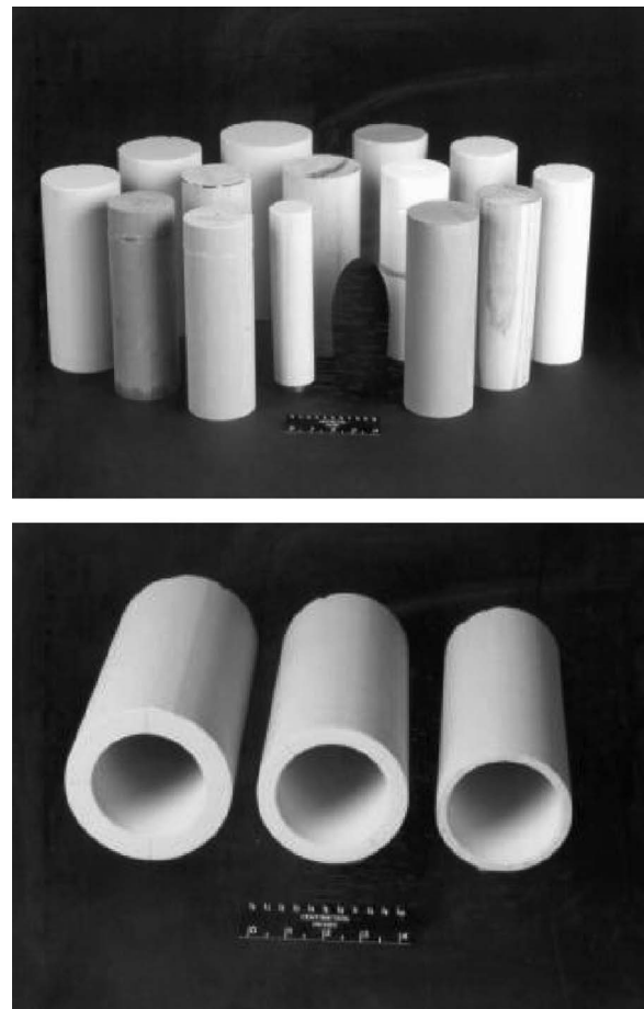
FIG. 3. Top: The family of tested windscreens. Bottom: View from the bottom of windscreens having an internal diameter of 0.0762 m (3 in.), internal depth of 0.23 m (9 in.), and wall thicknesses of 0.01905, 0.0127, and 0.00635 m ( \frac{3}{4} , \frac{1}{2} , and \frac{1}{4} in.), respectively. In service a windscreen is fitted with a bottom cap to accommodate the microphone.
